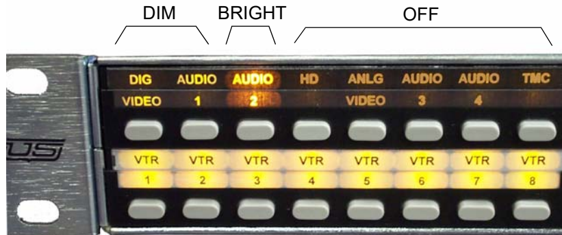
Figure 6-4. LED States of Illumination
